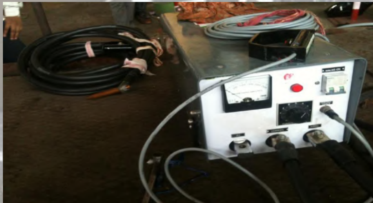
ITE's MPT equipment for Coil/Prod method
