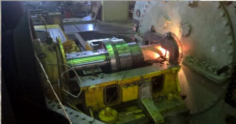
Bearing and oil inlet being inspected using Borescope
