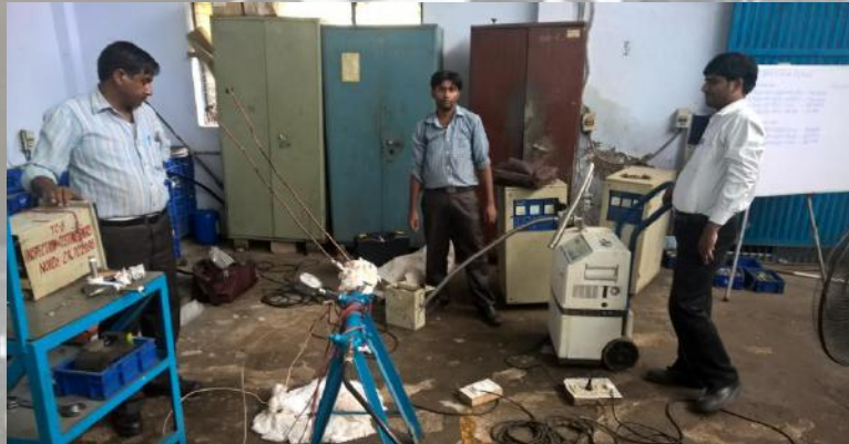
Fugitive Emission Testing of Valve using Helium Leak Detector
