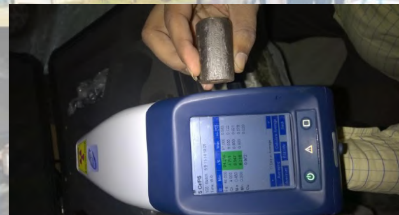
Positive Material Identification being done of Alloy Steel
