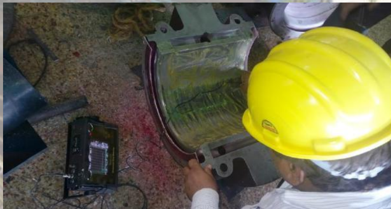
Ultrasonic Testing of Bearing being carried out
