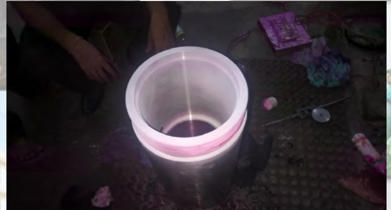
Visible Dye Penetrant Testing of Forged/Machined item
